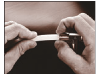
3. To disconnect push in collet and pull tubing
